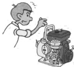
2. If the fuel level is low, fill to the shoulder of the fuel filter.
